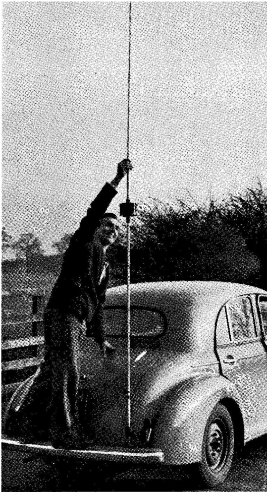
General appearance of the G3LIQ/M aerial as fitted. The method of construction, materials used and mounting ensure an assembly that remains steady under all normal travelling conditions.
